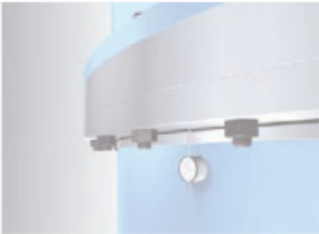
Fig. 28: Three-row roller bearing slewing ring – basic test setup for tilting clearance measurement
