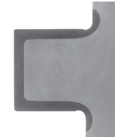
Fig. 15: Raceways of a nose ring in a three-row roller bearing slewing ring.
