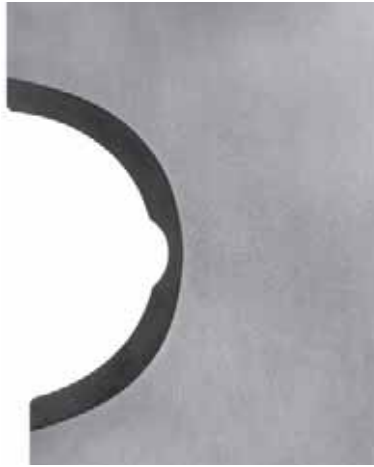
Fig. 13: Raceways in a single-row ball bearing slewing ring.
