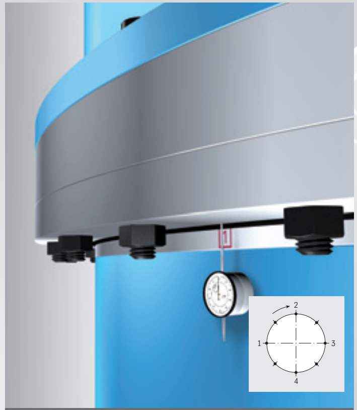
Figure 2: Basic setup for measuring the tilting clearance
